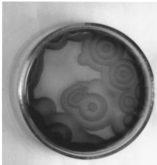
Figure 4. Pattern formation in the \text{BrO}_3^- -pyrogallol (PG)-DPA system. Initial concentrations (in M): \text{NaBrO}_3 , 0.0877; PG, 0.052; \text{H}_2\text{SO}_4 , 2.0; DPA 1.0 \times 10^{-4} .
